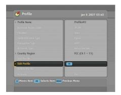
To make profiles for various network connections, select the Installation > LAN Setting > Profile menu.
